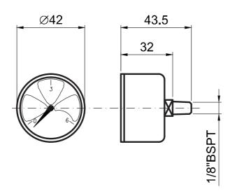
Visual or electric clogging indicators. Easy and cheap way of monitoring element clogging on our filters type SO, UCF, RTF, ect.
