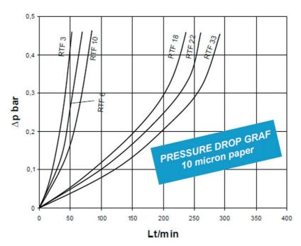
The graphics refer to mineral oil with a kinematic viscosity VG 46. The variation of the pressure drop is porportional to the kinematic viscosity
