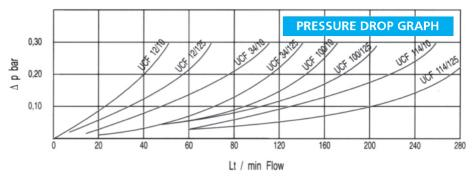
The graphics refer to mineral oil with a kinematic viscosity VG 46. The variation of the pressure drop is porportional to the kinematic viscosity
