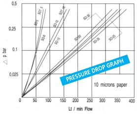
The graphics refer to mineral oil with a kinematic viscosity VG 46.
